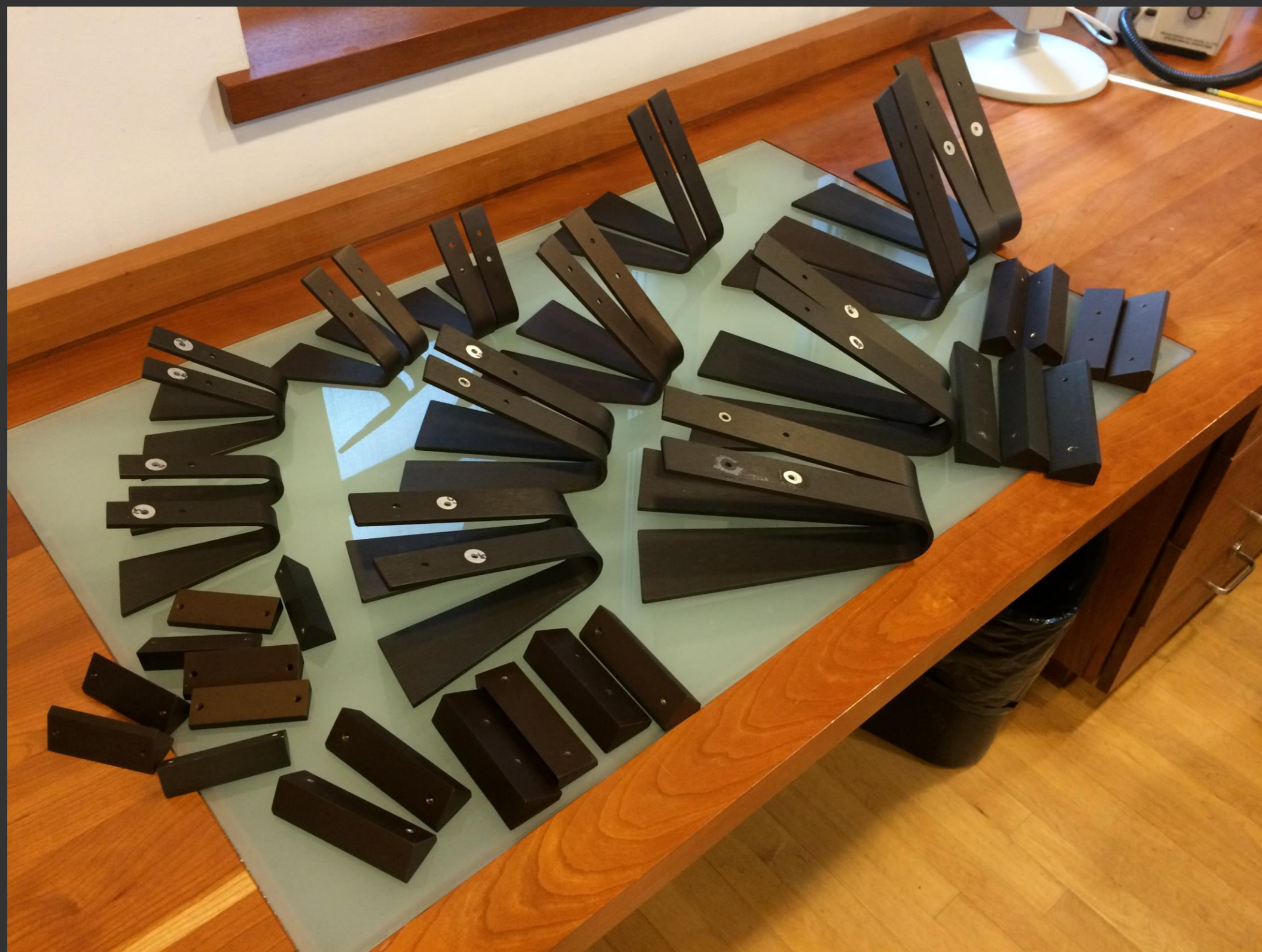
Brackets and cleats: Small, medium, large Four possible angles for tilt; combine angled cleats under book for safe opening
