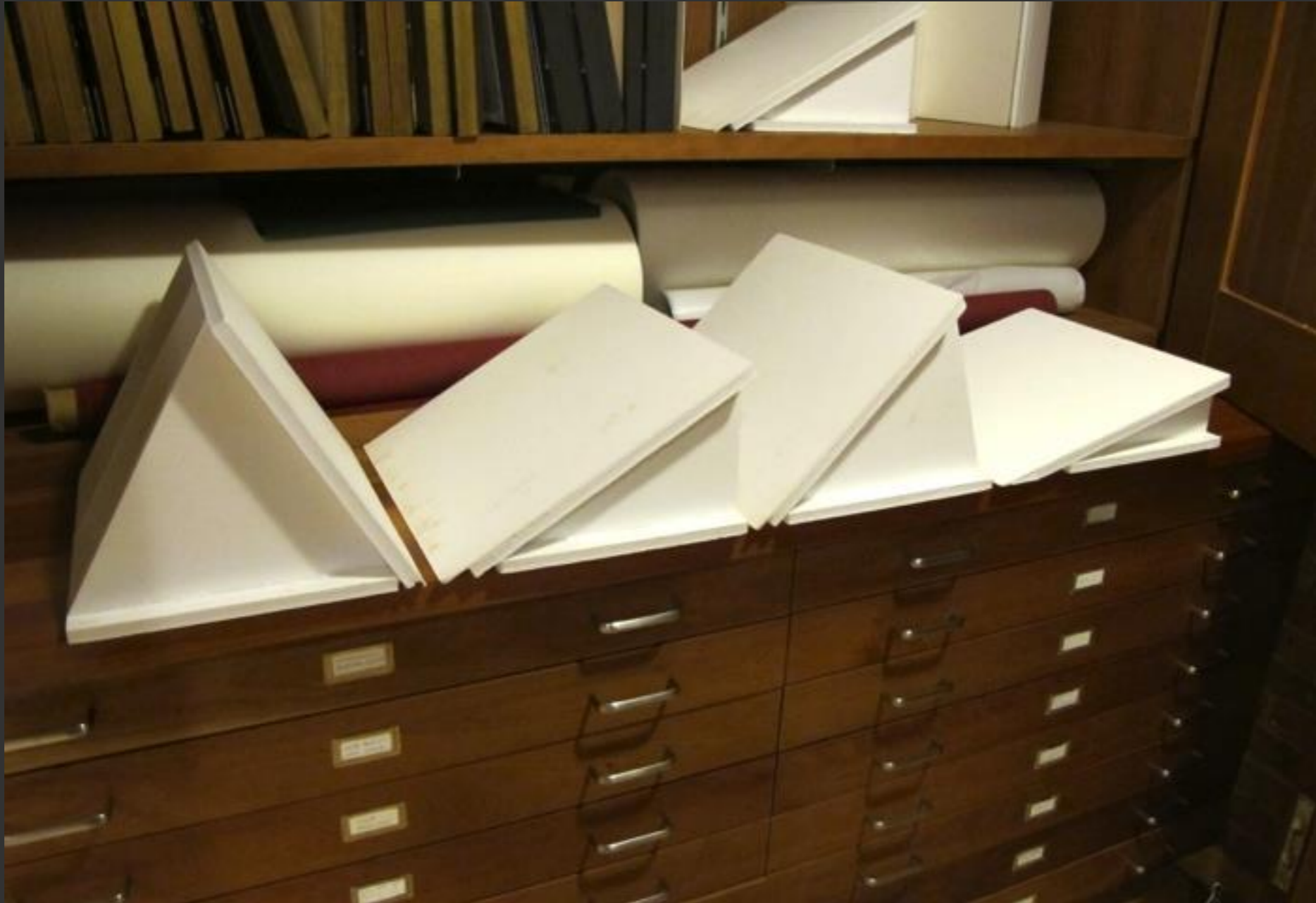
Foam-core wedges at 15, 30, 45 and 60 degrees; angles match metal cradle hardware
