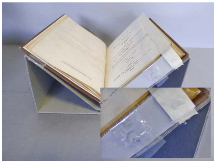
Figure 1. Adjustable page straps, made with embedded magnet and steel washer (inset detail), paper and polyethylene styles shown.
