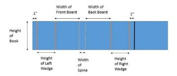
Figure 3. Placement of cuts and score lines for a basic cradle.
