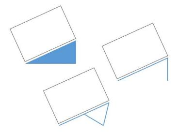
Figure 5. Options for a simple tilted cradle base.
